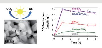
Fig. 1. High-entropy oxide with high photocatalytic activity for  $\text{CO}_2$  to CO conversion.
